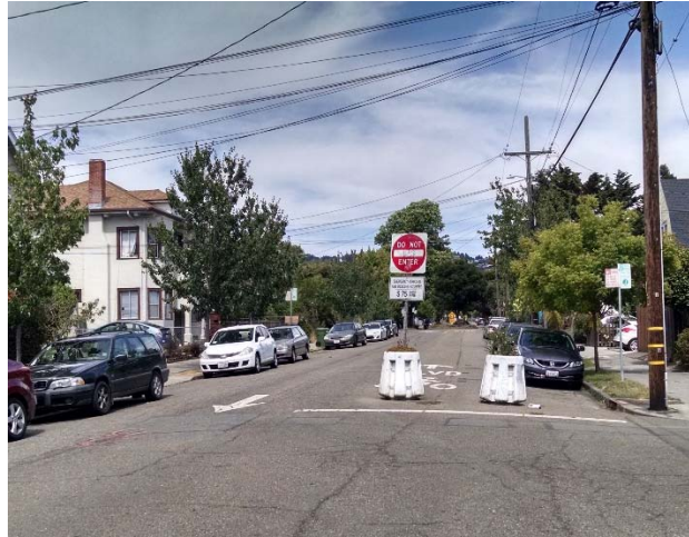
Figure 6 Partial Closure Example Russell Street, Berkeley, CA.
