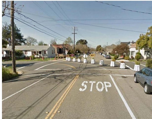
Figure 7 Traffic Diverter Example Berkeley, CA. Image: Google, 2017.
